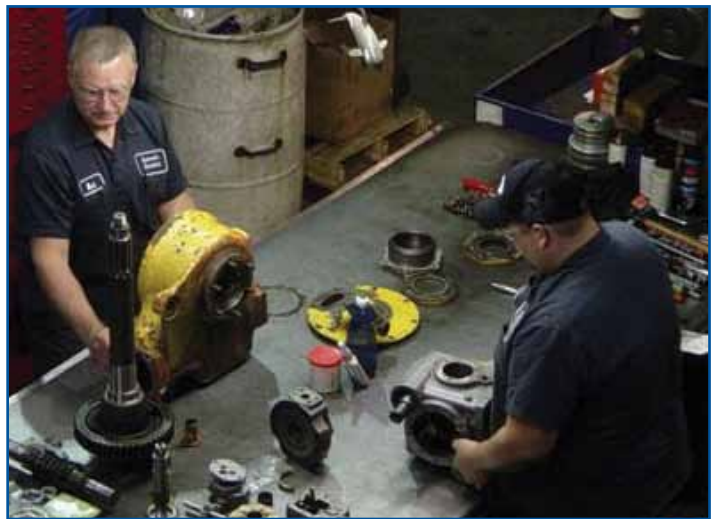
Hydraulic Pump & Motor Repair
